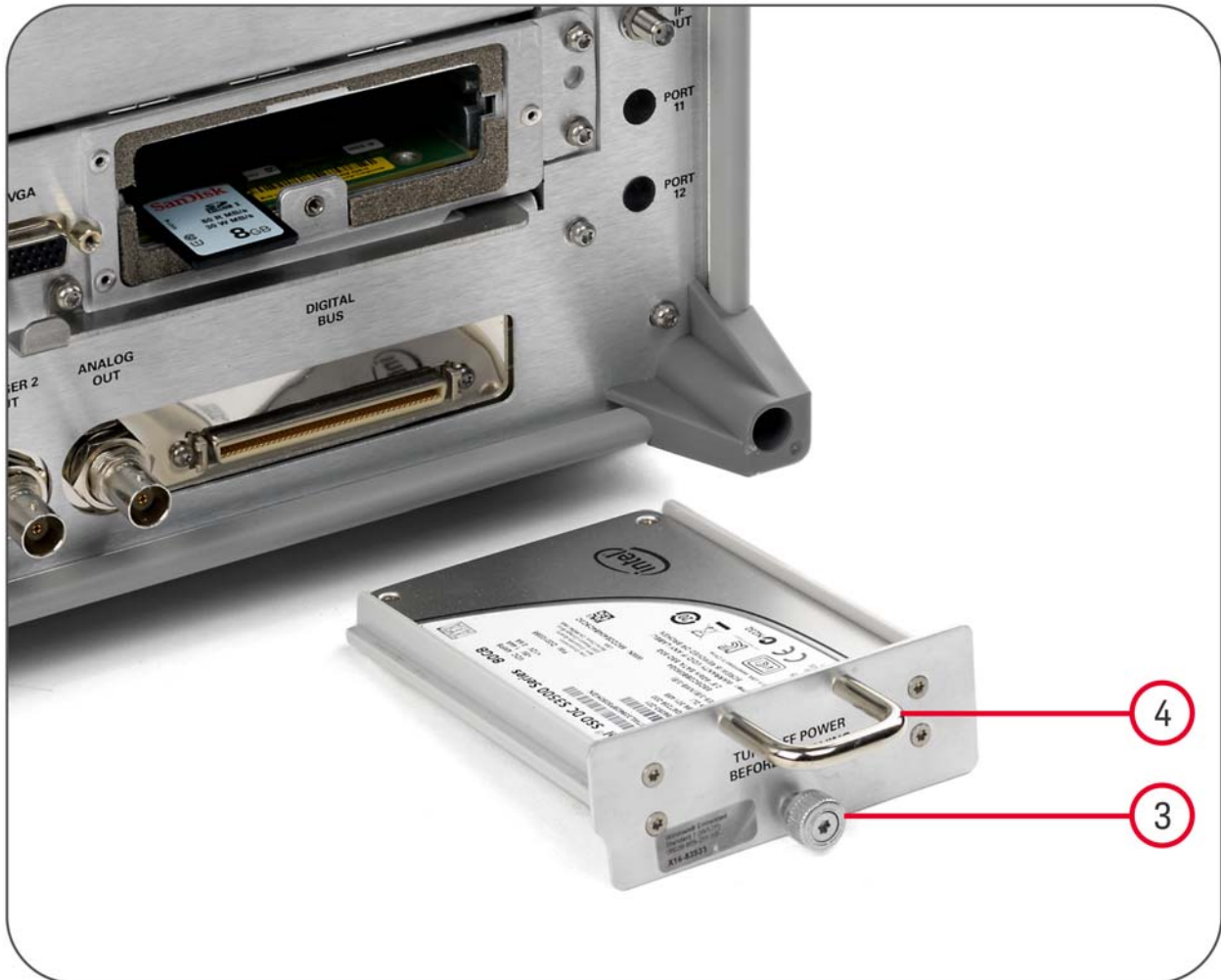
Figure 6-2 Removable Disk Drive Unit fully extracted
